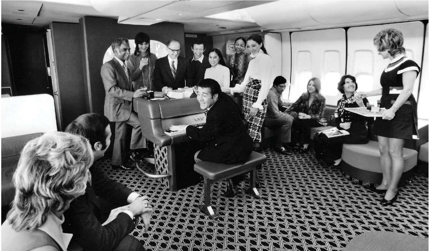
American Airlines eventually operated 19 747s, including two 747SPs, and installed Wurlitzer electric pianos in the coach class main deck seating zone 5 area on its early 747-100s. The pianos had truncated keyboards and were bolted to the deck.
