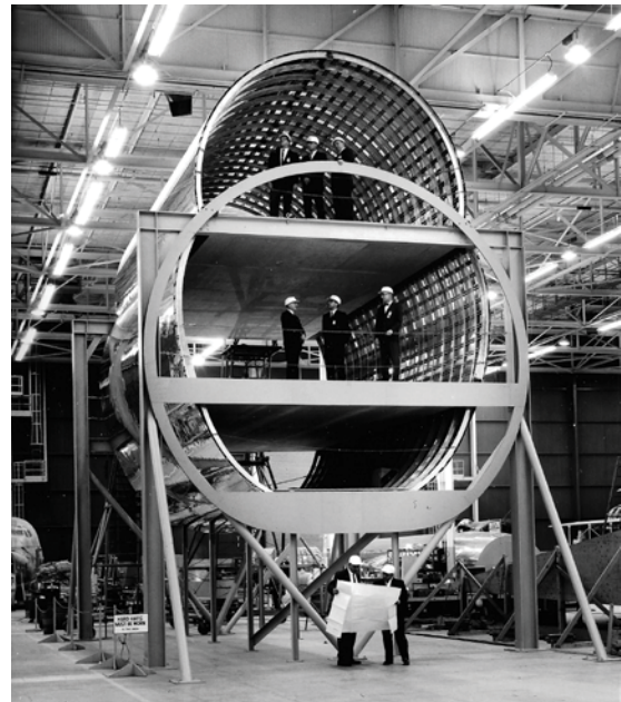
Early strands of the 747's DNA can be traced to the single deck mock-up of the CX-HLS airlifter.
